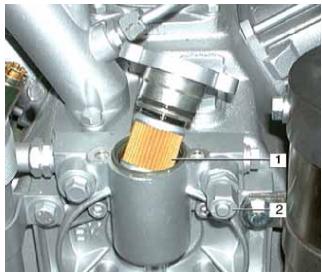
Figure 3-7 Replacing the Oil Filter
