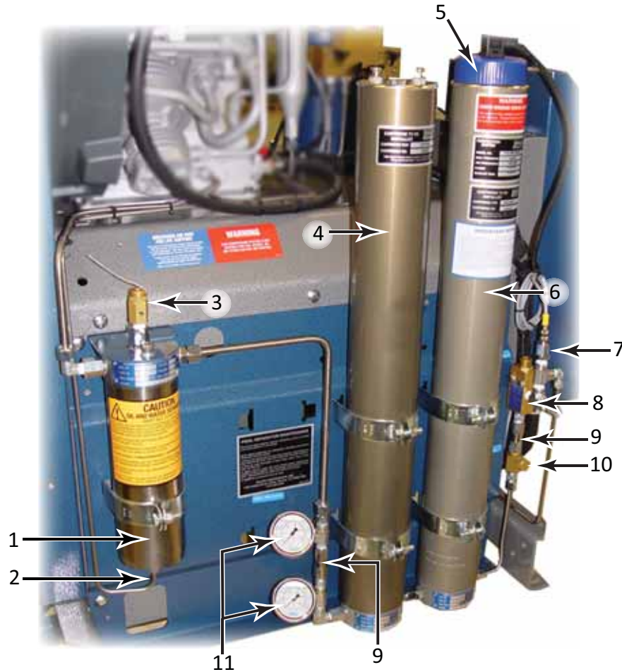
Figure 4-12 P5 Purification System Parts List
