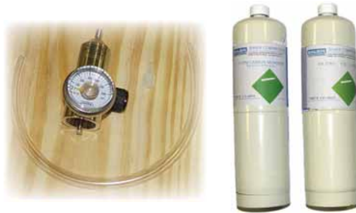
Figure 8-2 Basic Calibration Kit & Test Gases
